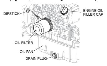
Figure 22. Engine Oil Service Components
